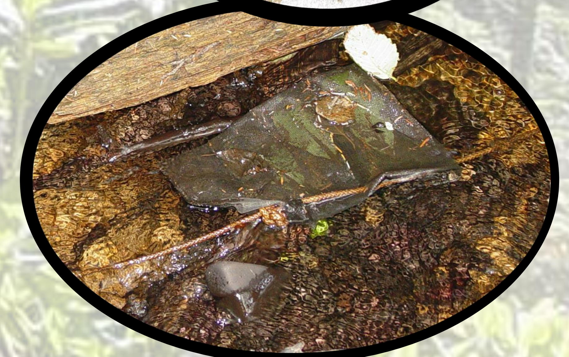
Figures 5 & 6 (above). Stream baiting bags filled with Rhododendron leaves used for Phytophthora ramorum aquatic detection.
