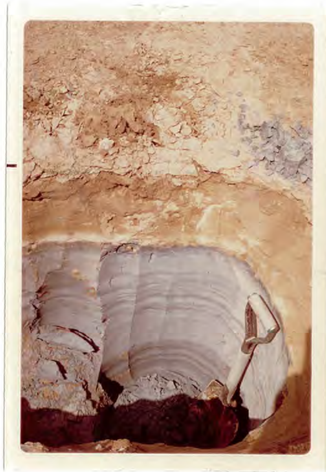
Photo No. 3. — Test pit dug 4 feet into tailings pile number 2 approximately 20 feet from a small central pond. The finer grained dark layers showed the glisten of surface moisture characteristic of "fat" clays but no water accumulated in the hole after 18 hours. The oxidized layer is about 10 inches thick. Note that there are no loose fines on the tailings surface but a "desert pavement" of iron oxide cemented chips.
