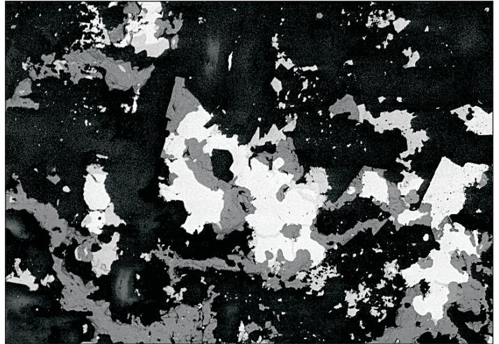
Figure G4. SEM image at 185x magnification of Knob Hill vein ore. Gold is white, quartz is black, chalcopyrite is light gray, naumannite is dark gray. The gold content over a wide field of view could not be estimated, but the silver content is approximately 13% by weight. Data and photo courtesy of G. Mustoe, 2009.
