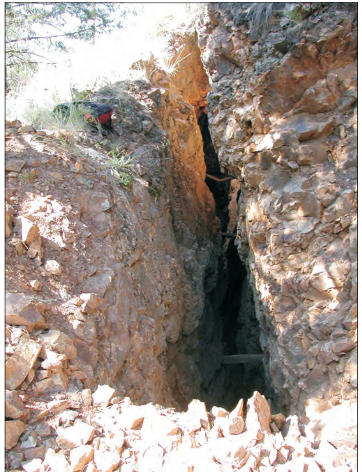
Figure 9. Open stope on the Lone Pine No. 3 vein. View downdip is ~200 feet. Pack at upper left for scale. View is to the northeast.
