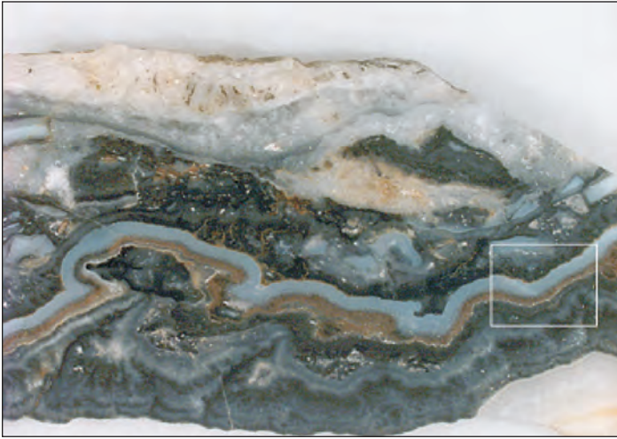
Figure G1. Polished Ben Hur vein outcrop sample showing black colloform chalcidony and quartz with minor calcite. Portion of insert pane is shown in SEM image below. Sample size is about 1.5 x 2 inches. Photo courtesy of G. Mustoe, 2009.
