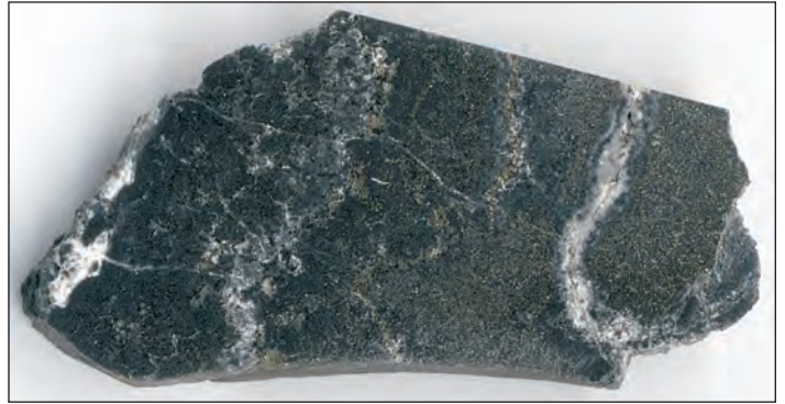
Figure G3. High-grade vein sample from the Knob Hill mine. SEM photograph below was taken in approximate center of the sample. Original size: 1 x 2 inches. Photo courtesy of G. Mustoe, 2009.
