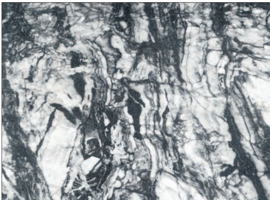
Figure 16. Colloform-banded chalcidonic veining in the Golden Promise mine. Dark bands contain most of the gold mineralization and metal sulfides. Area shown is 2 feet by 4 feet. (Reprinted from Derkey, 1996.)
