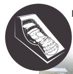
**Rotational slides** occur when rock or earth is transported downslope along a curved surface. This type of landslide can be large and damaging.
