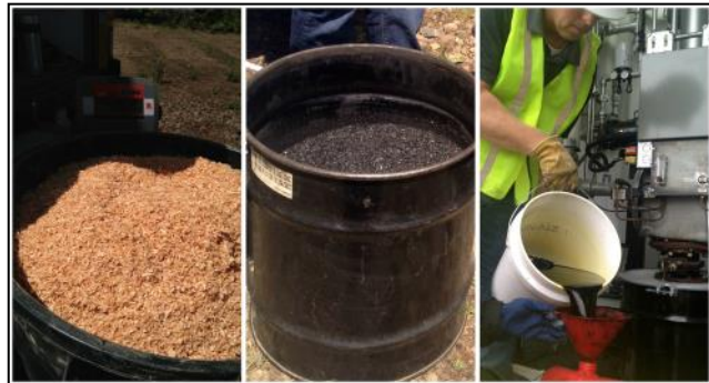
Figure 18. Douglas-fir planer shavings feedstock (left) converted into char (center) and oil (left) during Bingen, WA pyrolysis demonstration.
