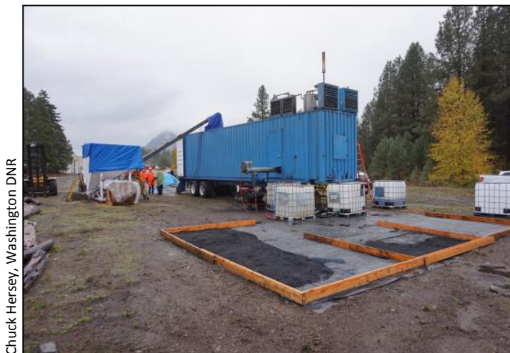
Figure 19. Amaron Energy's 20 ton/day mobile pyrolysis unit in Cle Elum, WA. October 2014. The white hopper with blue tarp on the left feeds wood chips into the pyrolysis unit, char comes out of the silver auger on the side of the unit, and oil goes to the white tanks. Char has temporarily been spread out in wooden pens to oxidize and cool.
