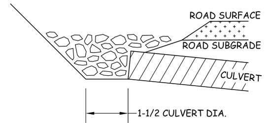
**CULVERT INSTALLATION WITH DOWNSPOUT**
