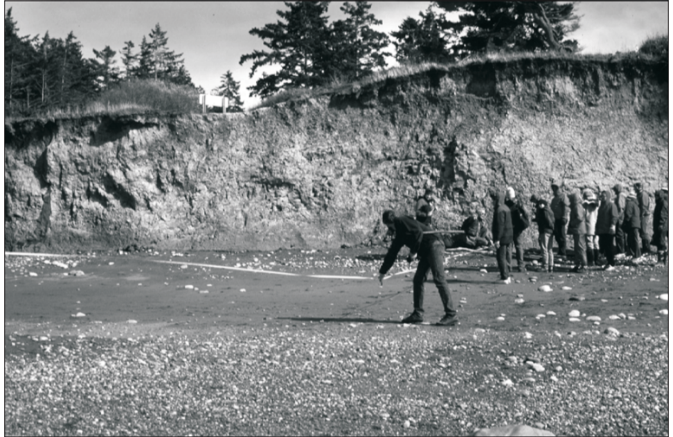
Figure 1. Volunteers learn to deal with one of the hazards of beach work—the wind. At this stop off Libbey Road, the challenge is to measure the distance from a certain point on a large boulder (just out of sight to the left) to a point on the bluff that they can revisit to determine if the bluff is retreating.
