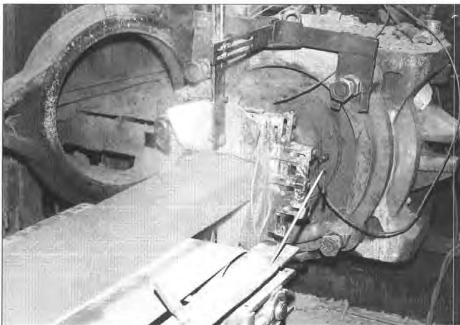
Figure 2. When the desired blend of source clay is reached, an appropriate amount of water is added. The clay is squeezed or forced into a mold from which it is extruded, in much the same way as toothpaste is squeezed out of its tube. The clay is extruded in a continuous stream onto a slowly moving conveyor belt. Different orifices are used to obtain the different sizes and shapes of bricks. If the design calls for holes in the brick, they are created at the orifice.
