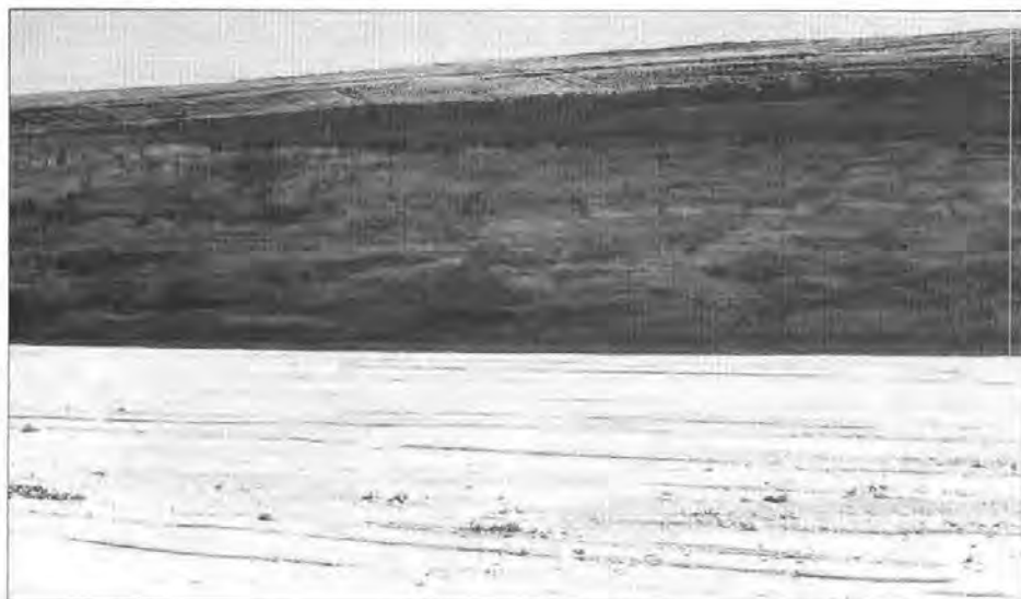
Figure 1. Highwall of clay pit. This is one of several pits where Mutual Materials Co. mines clay for making bricks at its plant in Mica, southeast of Spokane. The deposit contains about 65 percent clay, the remainder being quartz, feldspar, and mica. The non-clay fraction is about 65 percent quartz, 25–30 percent feldspar, and 5–10 percent mica. The pit highwall shown displays considerable color variation; the darker parts are stained by limonite, an iron mineral. By carefully controlling the mix of clays from this and several other pits, the Mica plant can produce a wide spectrum of brick colors.
