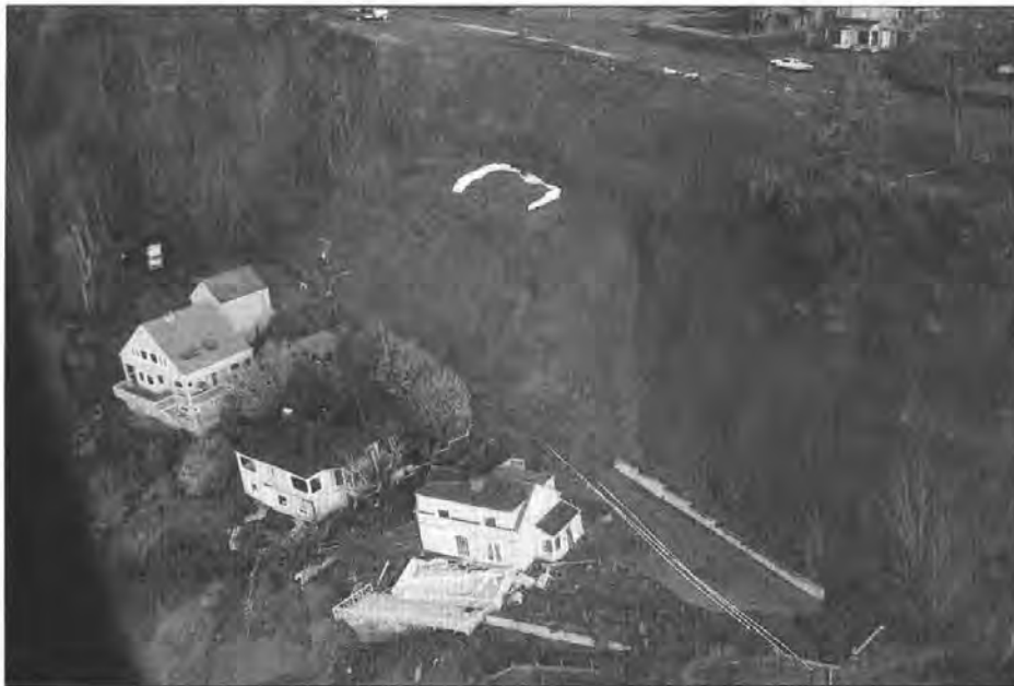
Figure 6. This photo shows one of the larger Seattle landslides along Perkins Lane on the southwest side of the Magnolia neighborhood. This is an area of continuing large-scale instability. Immediately following the February 1996 storms, a 1,500-yd 3 landslide (Harp and others, 1997) slid from the upper portion of the bluff into the back yard of the home on the right. Seattle engineers attempted to mitigate the problem by regrading and revegetating the upper slope. However, the February landslide was a shallow manifestation of a deep-seated rotational failure that formed, or might have already existed, in the sand, gravel, and silt deposits of the bluff at this site. This deep-seated slide was reactivated in December 1996, damaging at least five houses. These three are now uninhabitable. The white plastic sheeting on the slope was probably placed there in an attempt to prevent water from infiltrating the soil. This site is representative of the geologic conditions shown in Figures 20 and 21C.
