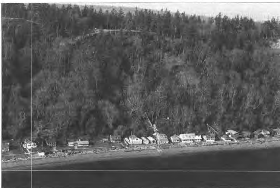
Figure 16. Several beach homes on the east side of southern Whidbey Island had close calls from debris avalanches. Debris avalanche tracks and deposits here will soon be colonized by alders. Stripes or patches of alder trees that are all of the same age can indicate areas where slide activity occurred in the past; the age of the trees indicates approximately when the slide(s) occurred. In the 1950s and '60s, many beach-level developments like this were constructed on fill behind bulkheads. Material for the fill was commonly hosed off the slopes or bulldozed from the bluffs. This may have contributed to continuing slope instability by destabilizing the toe of the slope.
