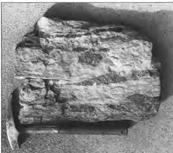
Figure 4. Sphalerite-bearing ore from northern Stevens Co. donated by Northwest Alloys, Inc., of Addy and displayed at the Keller Heritage Center, Stevens County Historical Society of Colville. There are several excellent rock and mineral collections in Washington.
