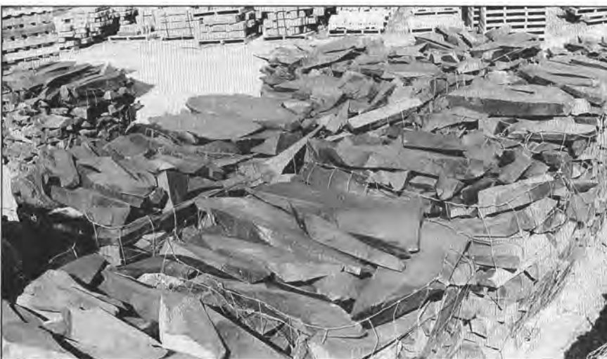
Figure 8. Palletized elongate pieces of “strip basalt” (also known as needle rock or liver rock) await installation as horizontal elements in a rock wall.
