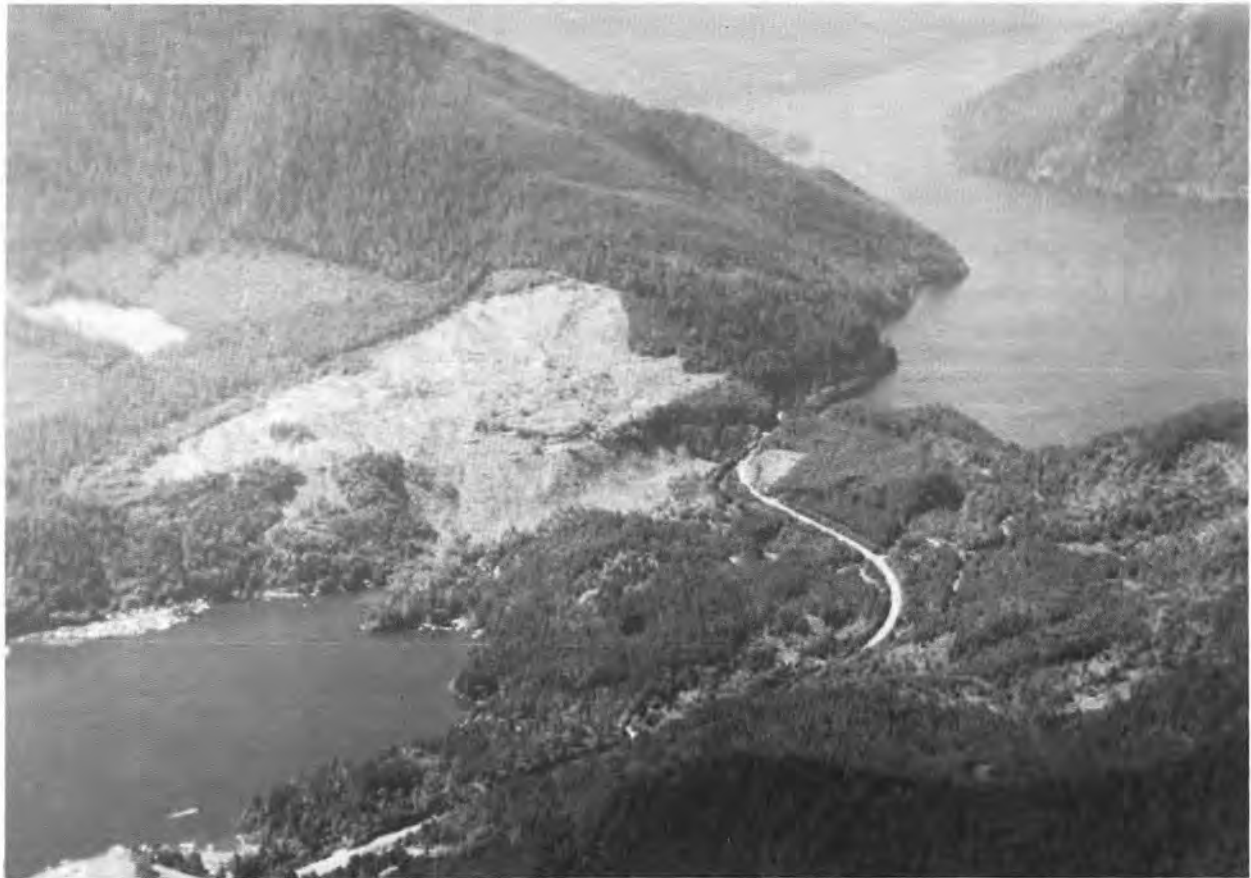
Lake Sutherland (foreground) and Lake Crescent, on the Olympic Peninsula; view to the west. Note landslide headscarps and the relative roughness of the surface of the landslide on the north side of the valley (right) beneath these scarps. (See article, p. 38.)
