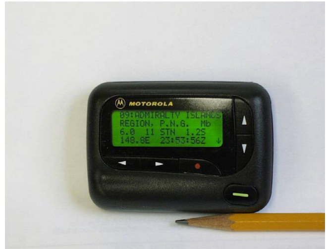
Figure 4. The pager photo shows what the on-duty person sees when an earthquake is automatically located and sized by EarlyBird and sent out to the pagers.
