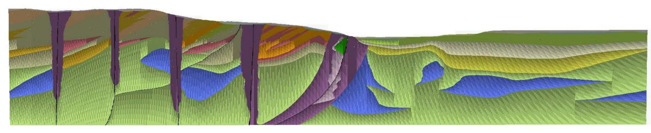
\*Cross section as viewed in ArcScene. Note the discretized segments are apparent due to ArcScene's renderer.
