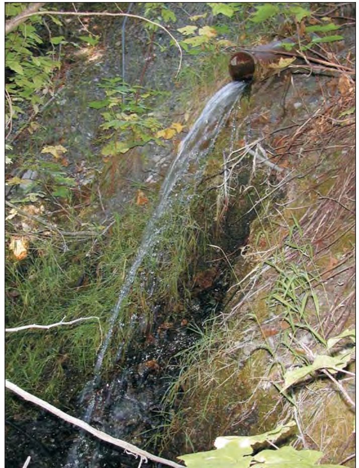
Figure 6. (bottom) Adit discharge at margin of waste rock dump.
