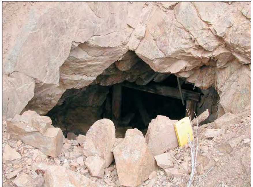
Figure 6. Sublevel drift that holes out into the open pit 40 feet above level 3 (Methow level). View to the west.
