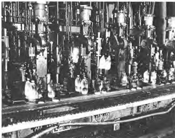
Bottle-making machine at Northwestern Glass Company, in Seattle. Bottles are red hot, which is why they glow. (Photo courtesy of Northwestern Glass Company.) Figure 45.
