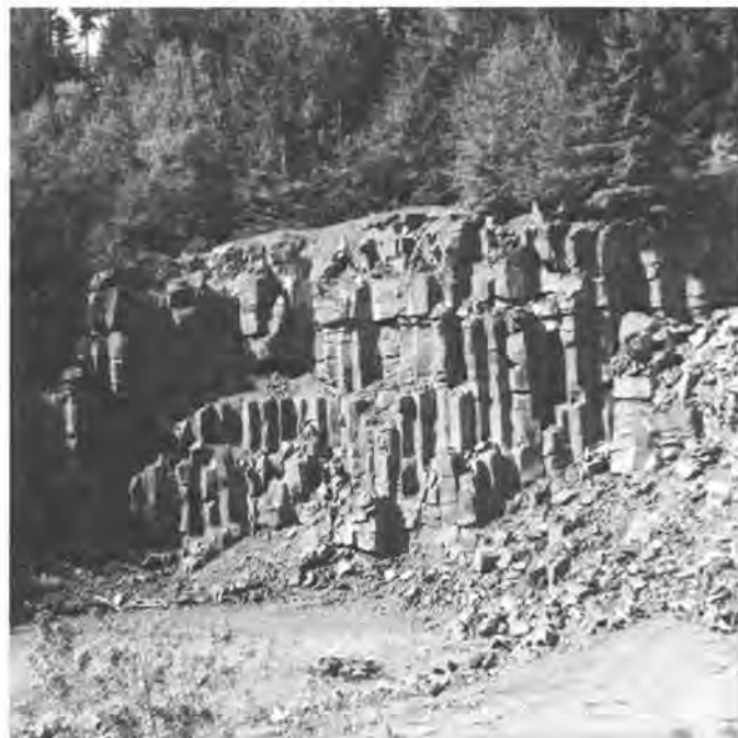
Columnar basalt near Longview, in Cowlitz County. The columns are quarried out in large blocks, which are used as riprap and in building jetties. Figure 37.
