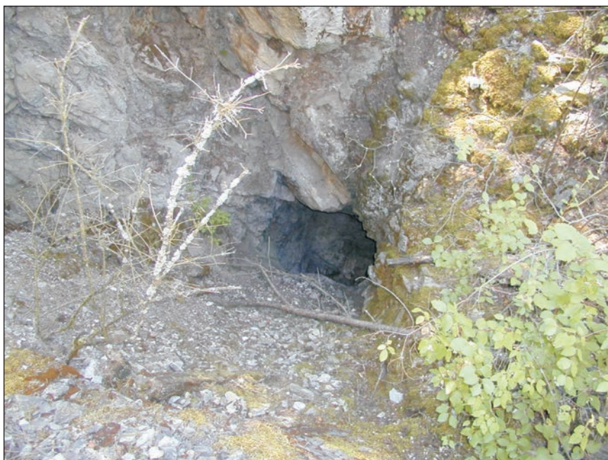
Figure 7. Unfenced winze dipping -65 degrees. View is to the southwest.
