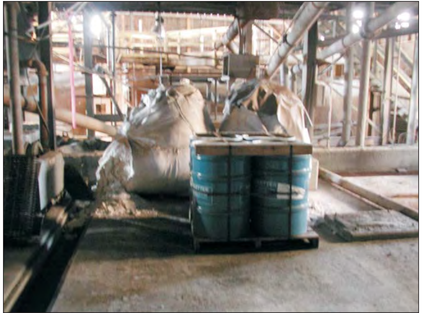
Figure 17. (top) Sodium carbonate (sacks) and copper sulfate (barrels) on mill bottom floor.
