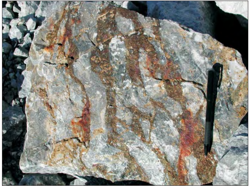
Figure 2. Streaks of sphalerite in dolomite. Pen for scale.
