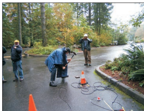
Geologist/cartographer Eric Schuster provides the seismic source by hitting a metal plate with a sledgehammer.
