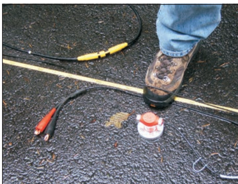
Staff members place geophones every 5 ft with the help of a tape measure.
