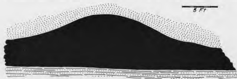
FIG. 8. No. 5 Mine, N. W. I. Co. Simple Roll in Roof on No. 1 Manway, East Side, Below 6th Level.
