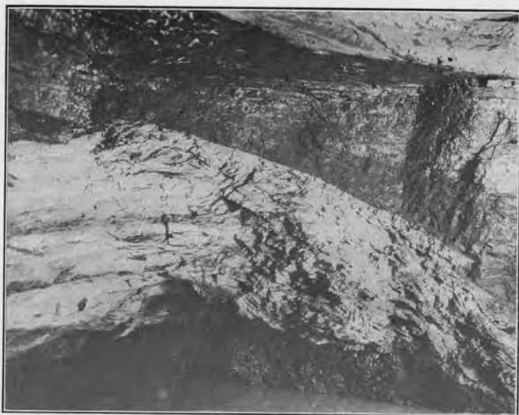
A. No. 5 Mine, N. W. I. Co. Detail View Similar to Plate XVIII Showing Change in Thickness of Coal and Roll in the Bottom Rock on 6th Level, West.
