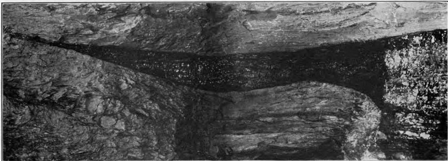
Pinching of the Coal on the 6th Level West at West End of Fault. No. 5 Mine, N. W. I. Co.
