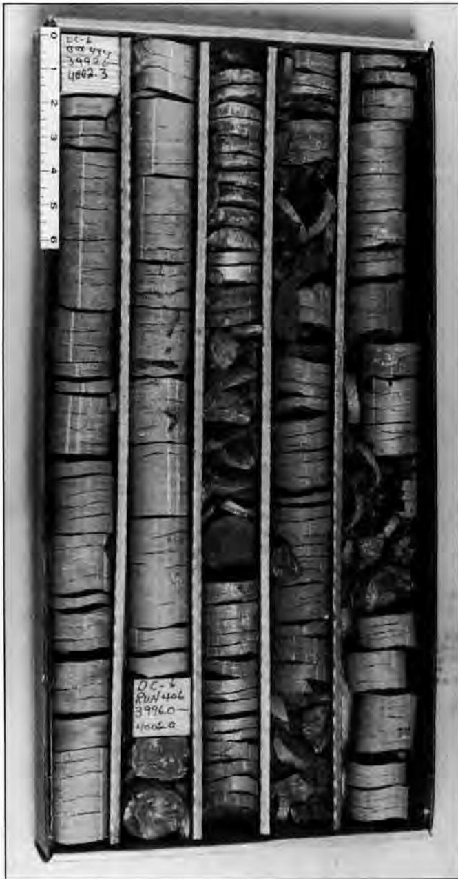
Figure 14. Disking in core, borehole DC-6, Hanford Site.
