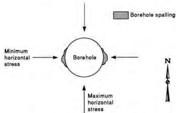
Figure 15. Generalized pattern of borehole spalling in the Cold Creek syncline. Redrawn from U.S. Department of Energy (1988).
