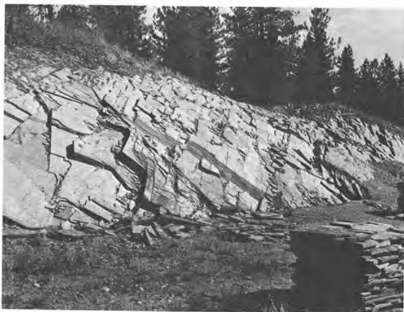
FIGURE 9. — Building stone quarry in quartzite. Note quartzite flagstones on pallet in lower right foreground.
