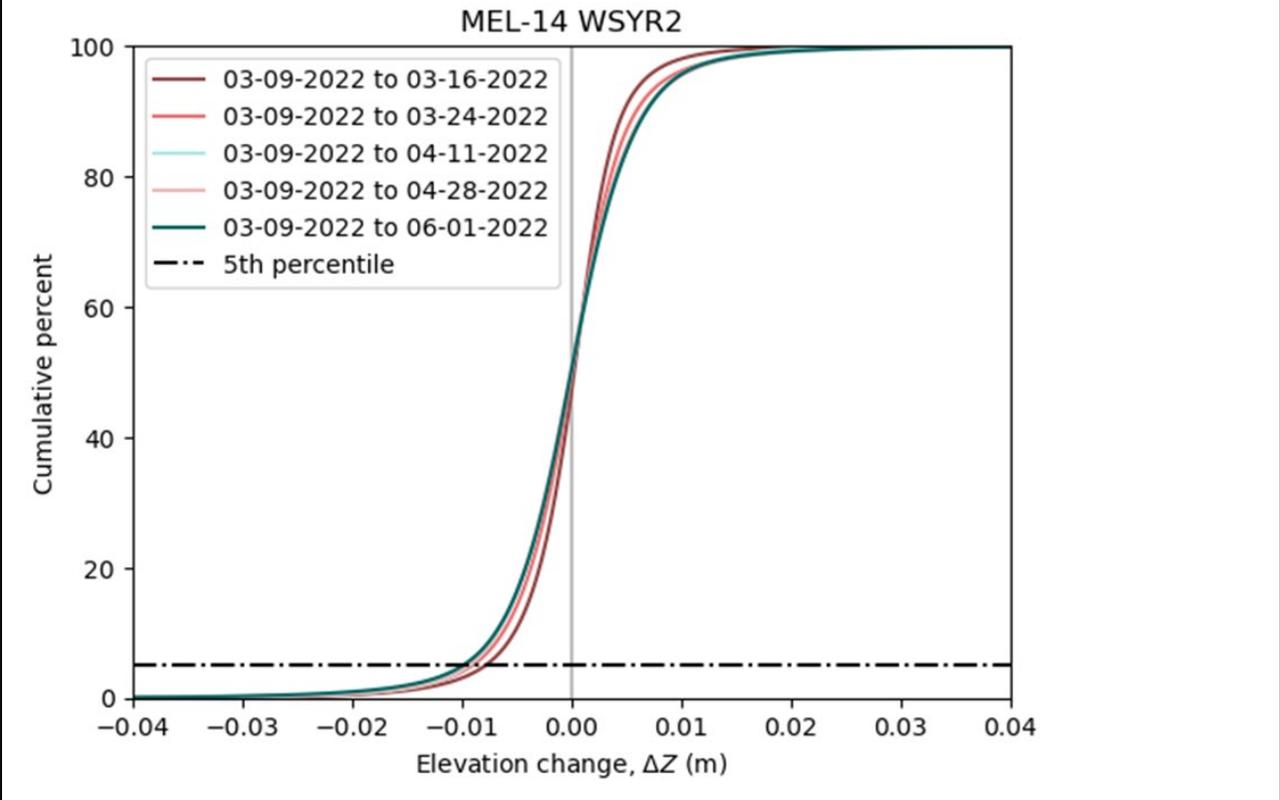
**Figure 5.** Example eCDF of elevation change for WSYR2 surveys at MEL-14.
