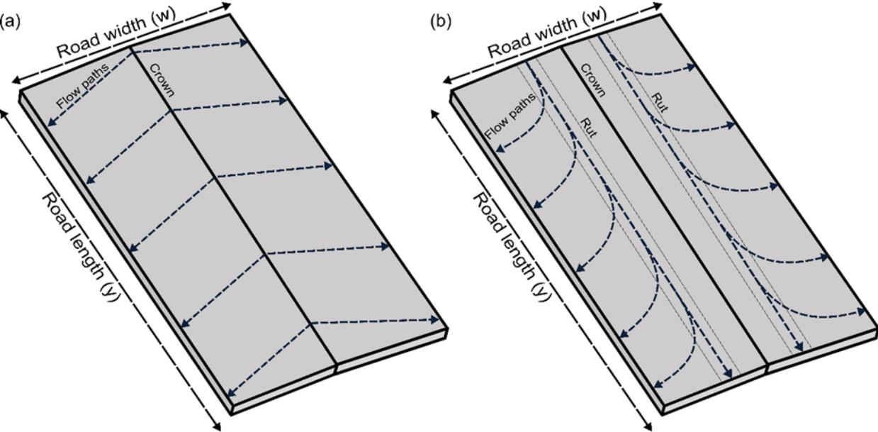
**Figure 7.** Schematic of a crowned road segment showing the flow pathways for (a) an idealized (i.e., perfectly smooth) road surface and (b) a rutted road surface.
