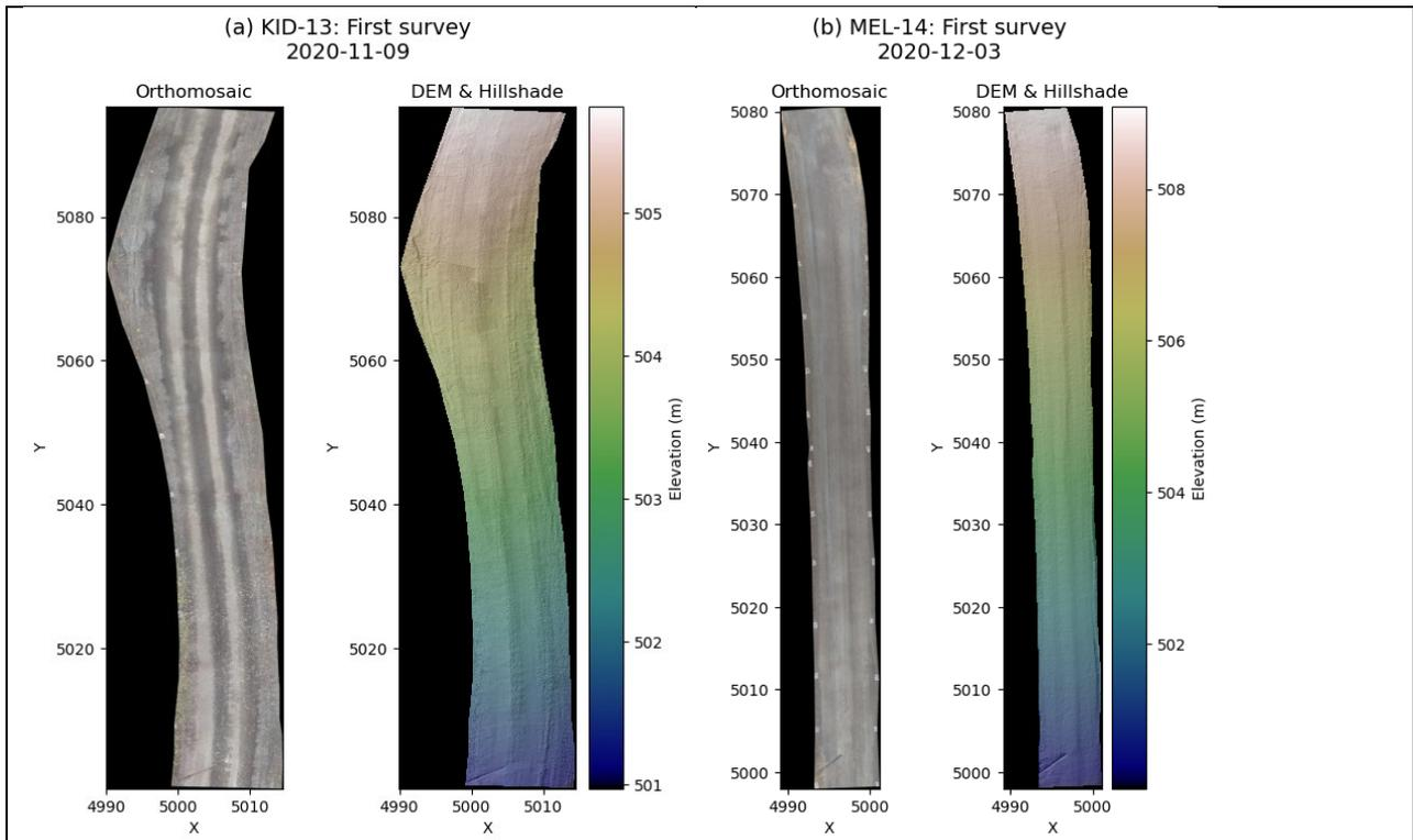
**Figure 2.** Example orthomosaic and digital elevation model overlaying a hillshade for the first survey at (a) KID-13 and (b) MEL-14.
