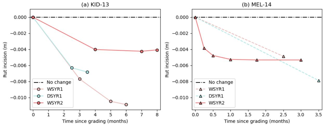
**Figure 8.** Plot showing the relationship between rut incision depth with respect to time since grading in months for (a) KID-13 and (b) MEL-14.
