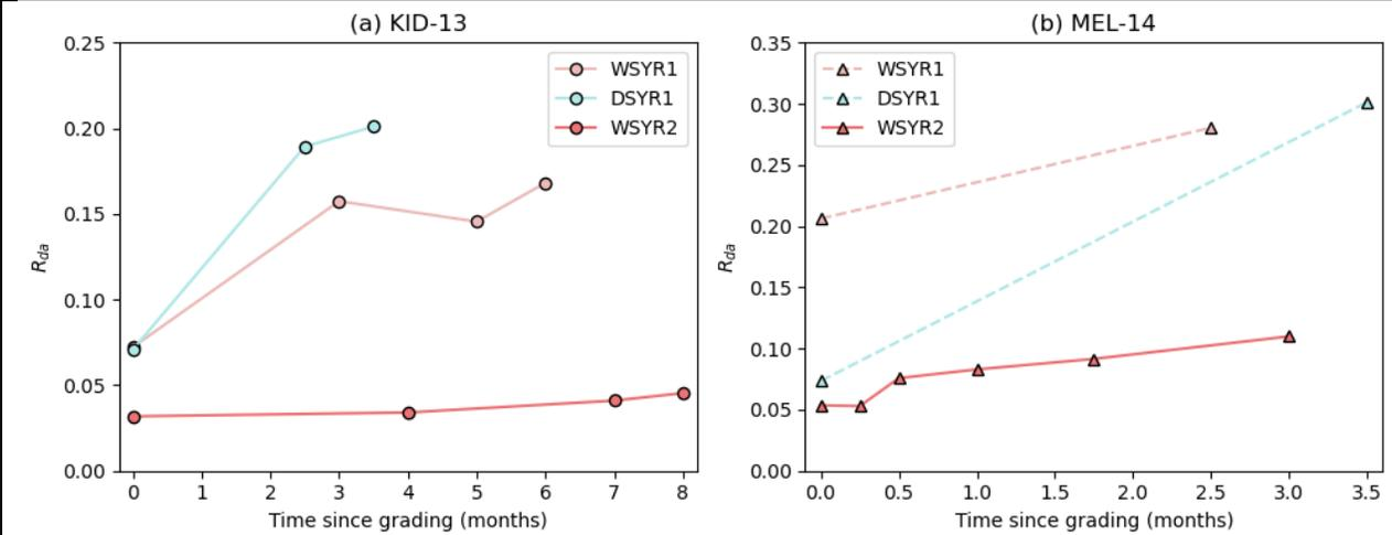
**Figure 10.** Plot showing the relationship between fraction of total drainage exiting through the lowest boundary of the road segment ( $R_{da}$ ) and time since grading in months for (a) KID-13 and (b) MEL-14.
