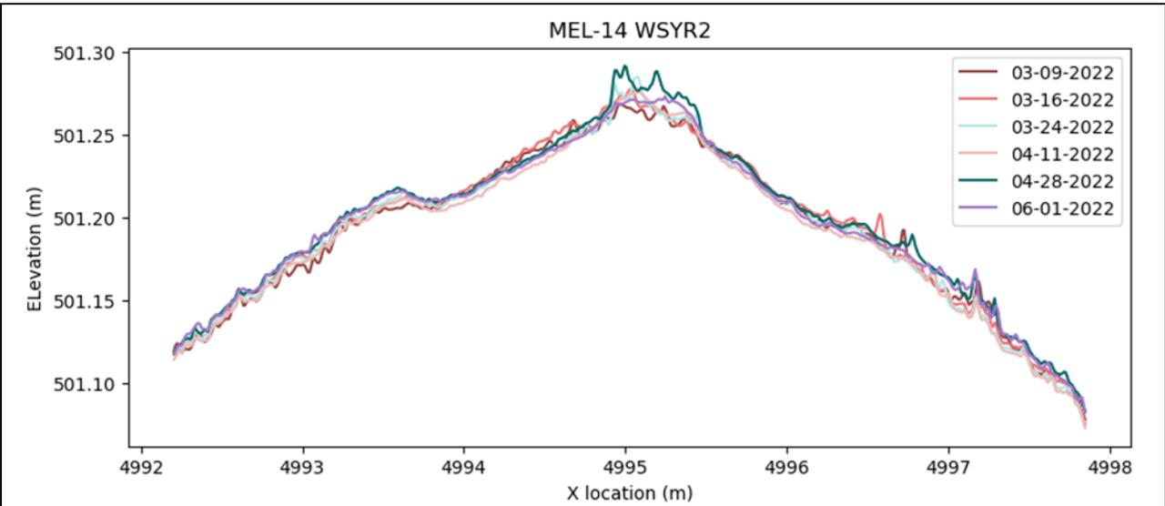
**Figure 4.** Example cross-sectional profiles of UAV-derived DEMs at MEL-14 for WSYR2.
