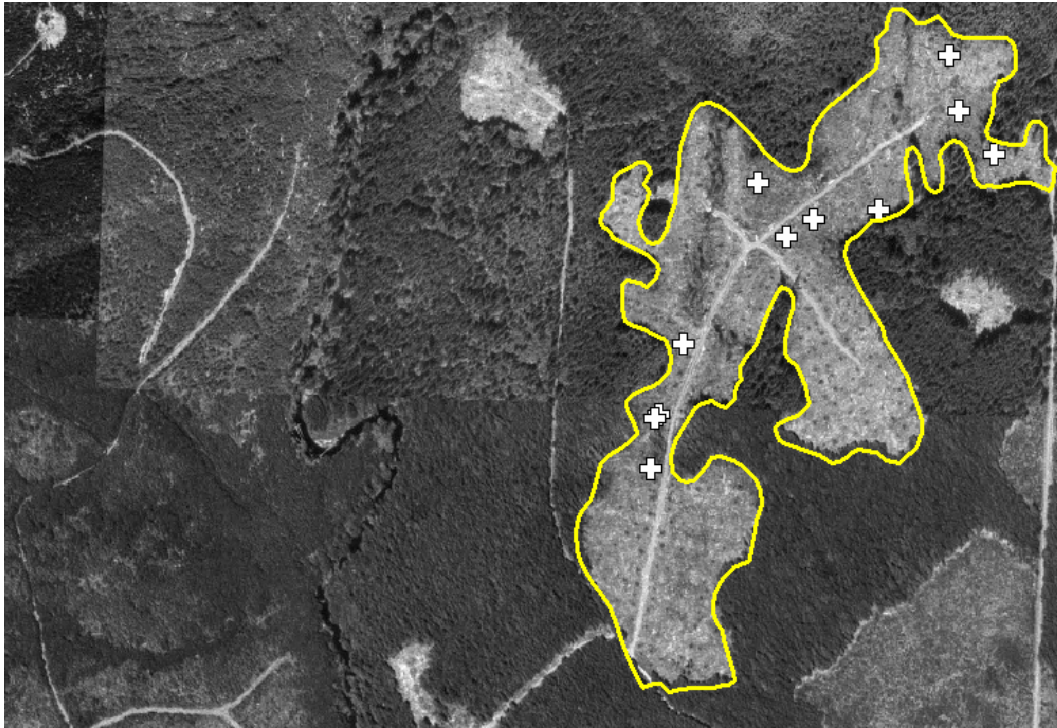
Figure 2. Sparse sampling. Outlined area was the harvest unit, about 56 acres. Eleven plots were scattered across this area, wherever the investigators found wetland conditions. This resulted in a sampling density of 0.2 plots/acre (scale=1:7000).
