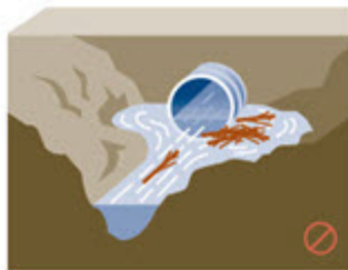
Figure 17 Design to prevent culvert plugging hazard
