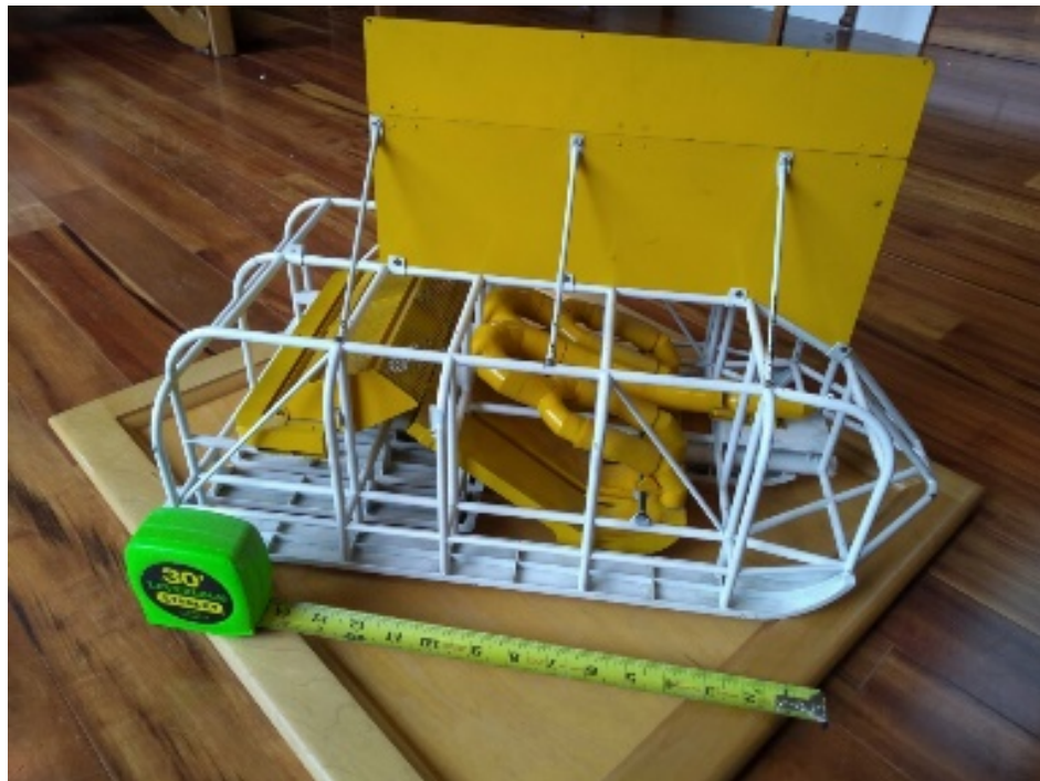
Figure 6 Physics of Eductors and model of multi-tasking Eductor sled
