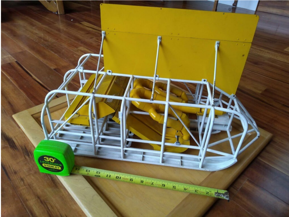
Figure 32 - Model of a deep water (13000 ft) eductor sled tested for manganese nodule recovery
