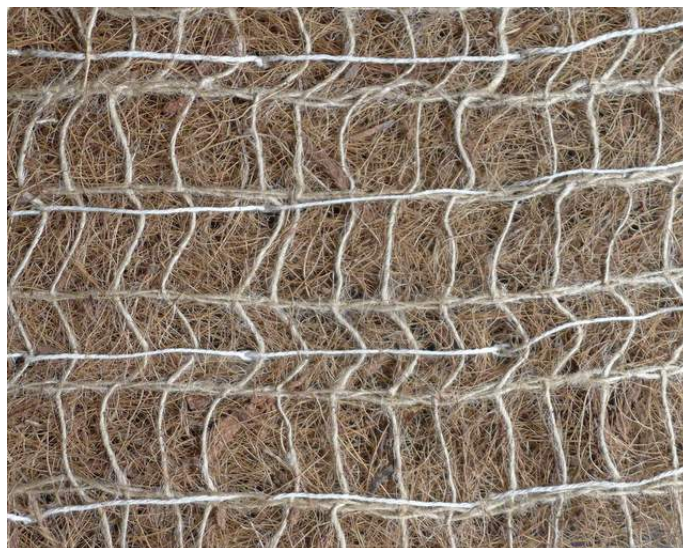
Figure 35 Coir Mesh: to be used as a middle layer of a composite mat
