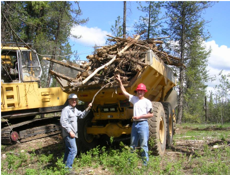
Figure 17. A load of low density harvest residue ready for transport to the main processing location
