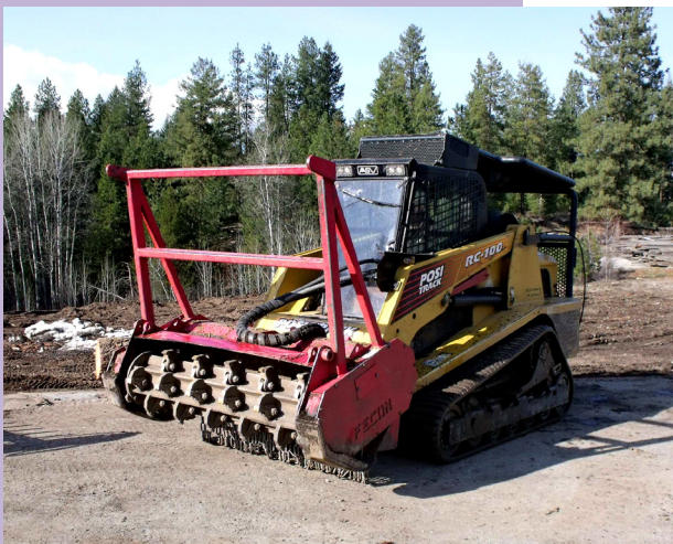
▲ ASV Skidsteer outfitted with a Fecon mulching head for stump and small material grinding, leaving the forest in a parklike condition.
