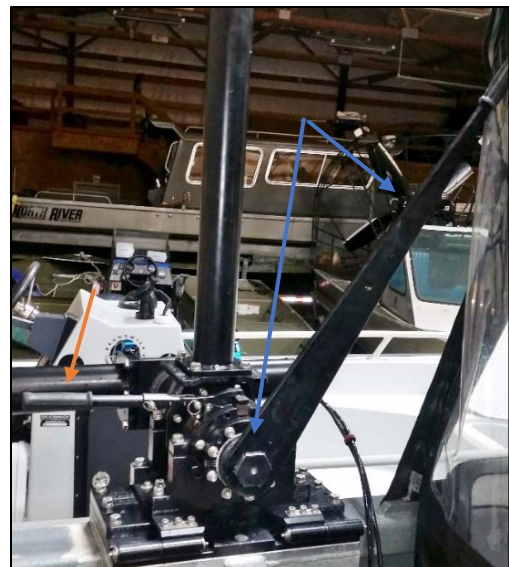
Figure 11: USM mounting X-pole in position to lower Z-pole in water
