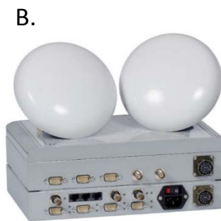
Figure 2. A. R2Sonic 2020 transducer, a POS MV and SVP mounted in frame. B. GNSS antennas and SIM
