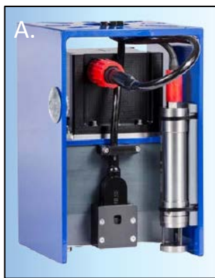
Figure 2. A. R2Sonic 2020 transducer, a POS MV and SVP mounted in frame. B. GNSS antennas and SIM
