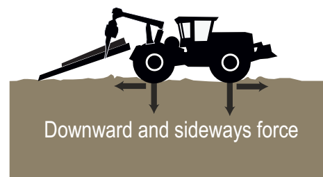
Figure 3-23. Soil Displacement; Skidder Shown
